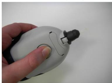
To release the probe press the button at the back and pull the probe out.
