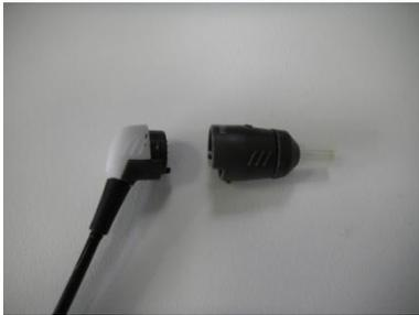
The probe can be attached to the extension cord by lining it up correctly and clicking the probe into the end of the extension cord.
