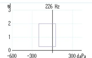
Here you find the graphics of the ongoing test. The box indicates the normative area where the peak of the tympanogram is expected under normal conditions.
