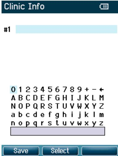
Use Up, Down, Right and Left arrow keys to move the cursor over the keyboard. Top middle button will select the highlighted character and put it where the cursor is placed. Backspace is found as an arrow in the top right corner. Space is found as a bar underneath the keyboard. Top right button will select the next details for editing. Top left button to save and return to the Setup screen.
