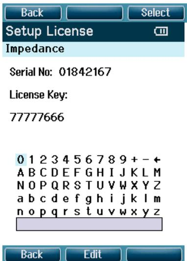
Use Left, Right, Up and Down arrow keys to move the cursor over the keyboard. Top middle button will select the highlighted character and put it where the cursor is placed. Backspace is found as an arrow in the top right corner. Space is found as a bar underneath the keyboard. Top right button will select the next details for editing. Top left button to save and return to the Setup screen
