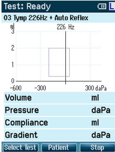
Usually the easyTymp starts with the Test Screen. When deleting or saving data after a measurement, you will also return to this screen. The following information can be viewed in the screen
