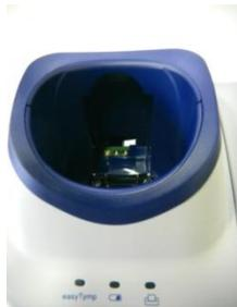
The spare battery is stored in the charger in the back of the cradle. Battery LED shows solid blue when the spare battery in the cradle is fully charged. The LED will flash as long as the battery is charging
