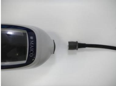
Place the probe to the easyTymp by lining up the red triangles and pushing the probe into the unit.
