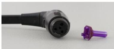
Place the probe tip back onto the probe. Make sure that the different holes fit in the corresponding cavities.
