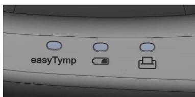
**easyTymp LED** shows solid blue when the easyTymp is placed inside the cradle and the battery is fully charged. The LED will flash as long as the battery is charging.
