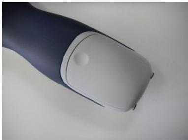
The battery compartment is opened by gently pressing the indentation and pulling the cover downwards.
