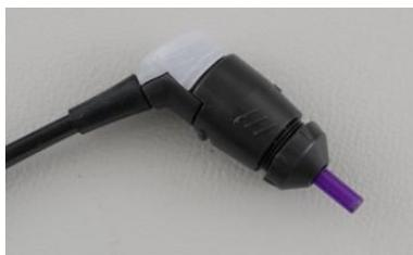
Screw the probe cap back on the probe. Finger force will tighten the screw sufficiently. Never use tools to fix the probe cap!
