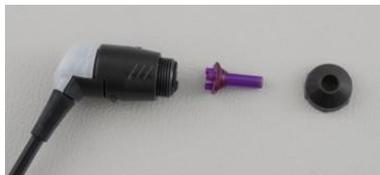
Take the probe tip out of the probe.
