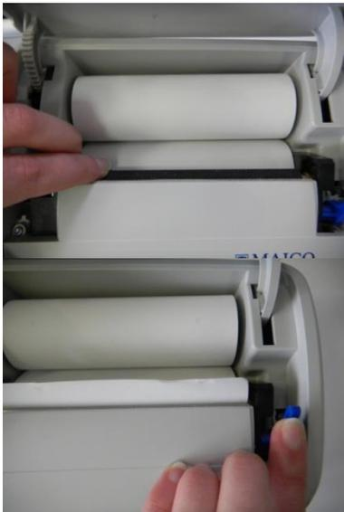
Insert paper roll in the compartment with its loose end to the front of the printer. Position the loose end into the printer roll and hoist it by rotating the printer roll with your finger
