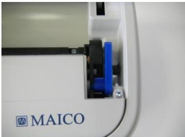
Step 2 – Pull blue lever upwards
