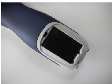
Place the battery inside the compartment. Make sure the battery contacts are correctly placed.
